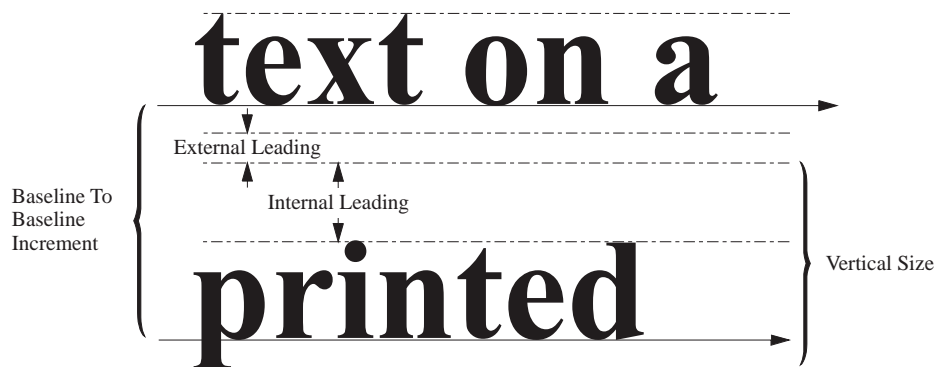
Figure 36. An Illustration of External Leading
