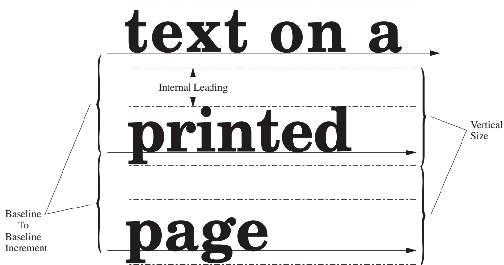
Figure 35. An Illustration of Vertical Size and Internal Leading
