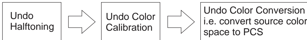
Figure 5. Procedure for Converting Input Data to Full Color in PCS
